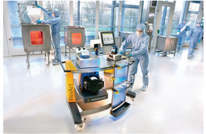
Figure 6. Portable Single Use System (SUS) based unit operations can be configured to perform a variety of processing steps ( photo courtesy of Sartorius ).
