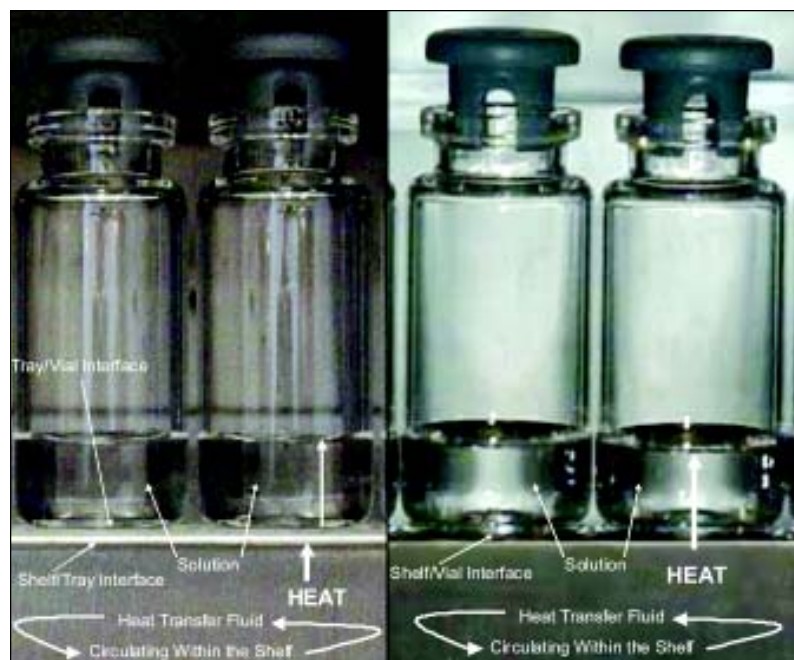
Figure 1. Heat transfer from the shelf to the product using a bottomed tray (left) and a bottomless tray (right).
