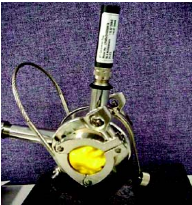
Figure 2. Calibration is inline, non-invasive, accurate, with no stoppage of water flow. Calibration unit is mated to the conductivity sensor as shown above.
