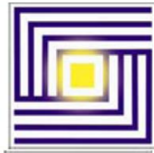
Incomplete air removal, Leak in autoclave
